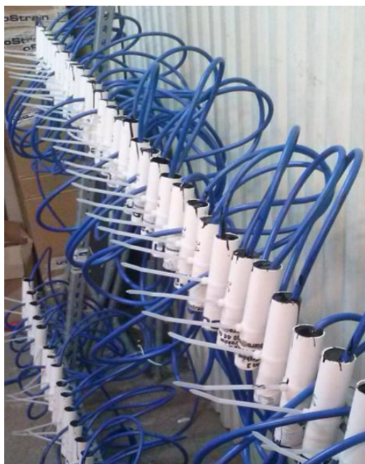
Fig 3. MCableS © multipoints temperature measurements cable (fot. Neostrain).
